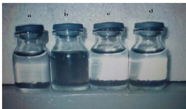
Figure 4 Photos of the MWCNTs in DMF, respectively, (1 mg for each kind of nanotube dispersed in 15 mL of DMF). (a) unfunctionalized MWCNT, (b) DDA-MWCNT, (c) EDA-MWCNT, (d) TETA-MWCNT. [Color figure can be viewed in the online issue, which is available at wileyonlinelibrary.com .]
